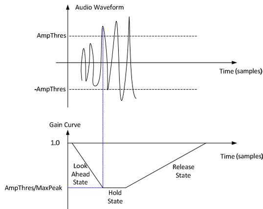
Figure 2 LIM Gain Curve for Linear Interpolation Approach
