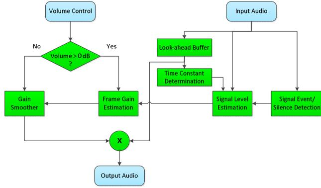
Figure 1 The Proposed Data-Driven Open-Loop AVC Alg.
